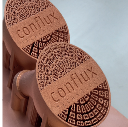
Fig 2: CuCP demo part (AMCM M 290-1 1kW). Source: Conflux technology
