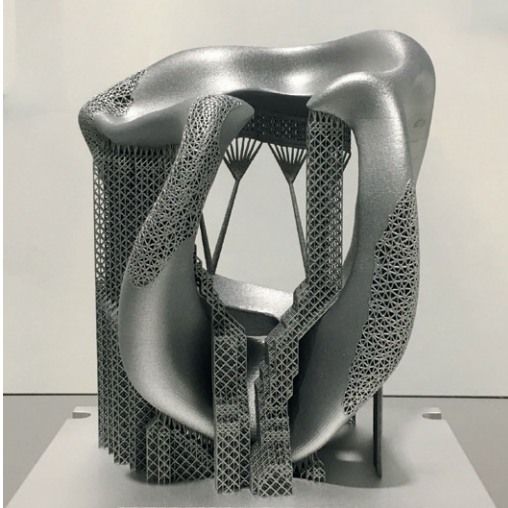
Fig 1: AlSi10Mg demo part manufactured in segments with dynamic adaptive parameter sets (AMCM M 290-1 1kW). Volume rate: 12 up to 32 mm 3 /s Source: EOS Innovation Center Düsseldorf
