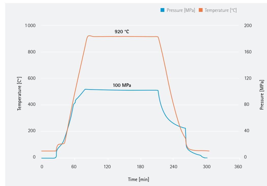
Figure 7a: Standard HIP cycle for titanium alloys (920 °C, 100 MPa, 2 h)
