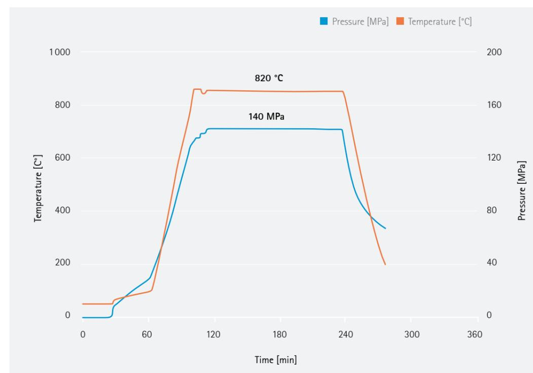
Figure 7b: Optimized HIP cycle for LPBF Ti64 (820 °C, 140 MPa, 2 h)
