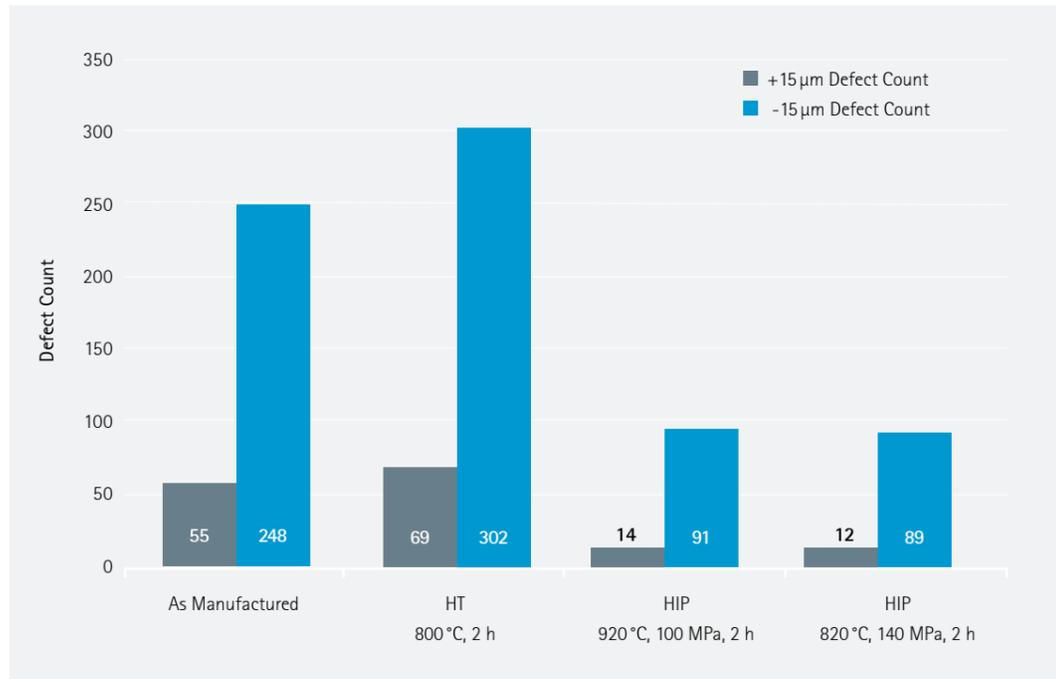
Figure 10. Defect analysis of as-manufactured, heat treated and HIPped LPBF Ti64
