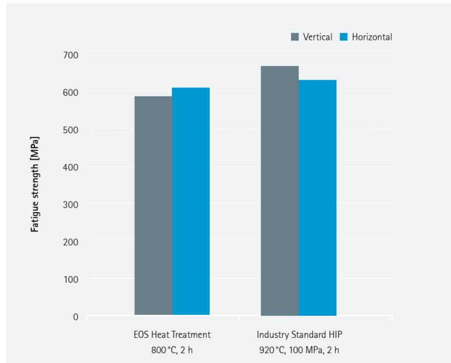
Figure 2. Fatigue strength ( $10^7$  cycles) of EOS Ti64 HiPer 40  $\mu\text{m}$  material in heat treated state and HIPped with industry standard parameters show only a minor difference
