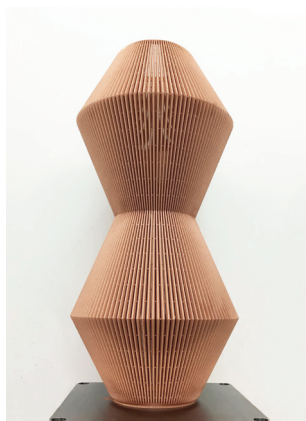
Fig 2: CuCrZr demo part The first ever 1,000 mm CuCrZr AM part, system: AMCM M 4K-1 1kW
