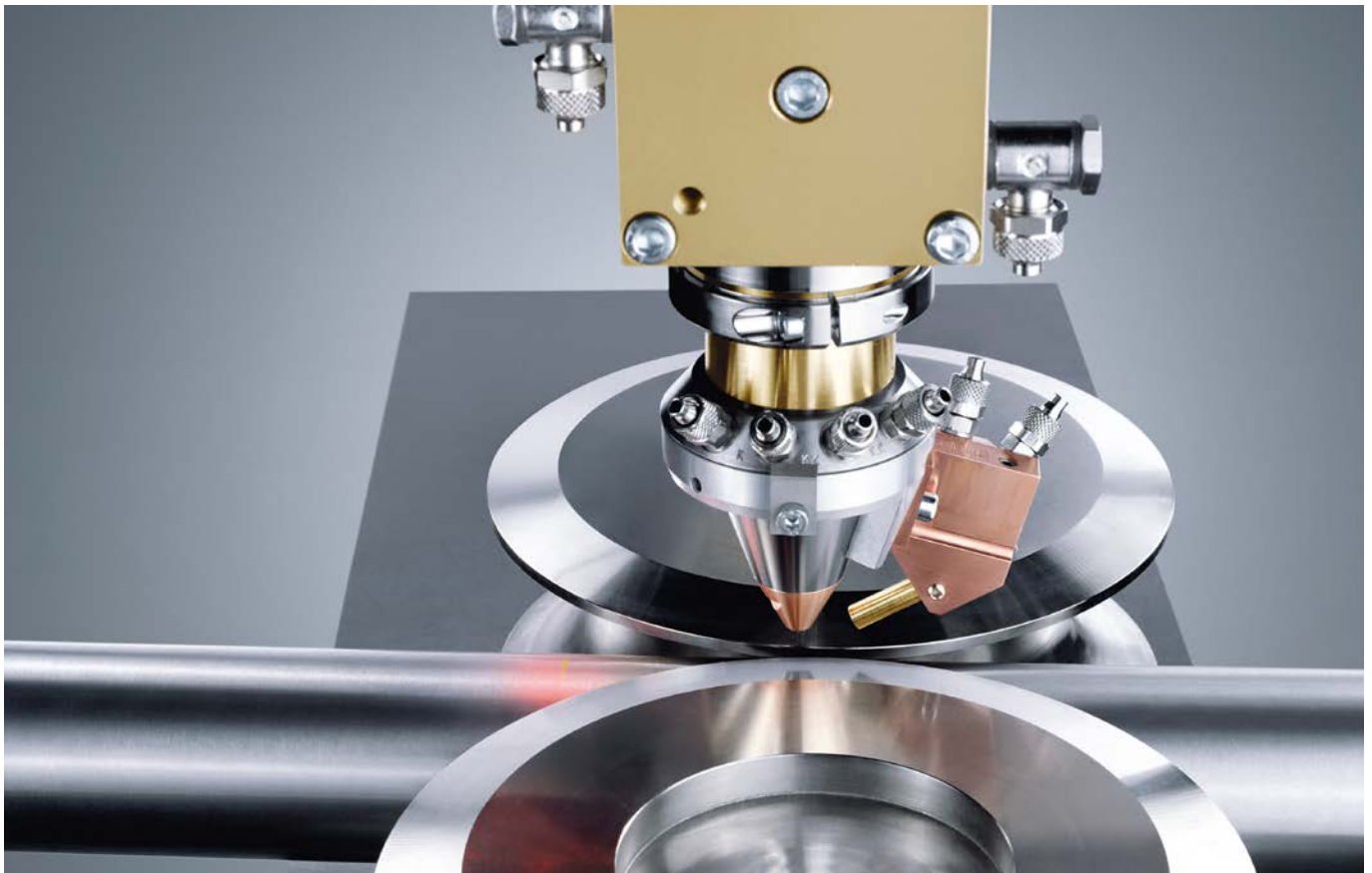
Continuous welding of tubes.
