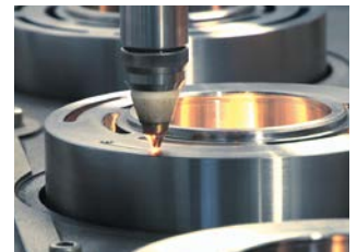
Laser cutting the housing of a water pump clutch.
